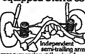
Independent semi-trailing arm rear suspension strikes just the right balance between sporting handling and a comfortable ride.
